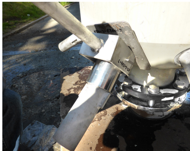
A special tool for taking out the ejector arms
